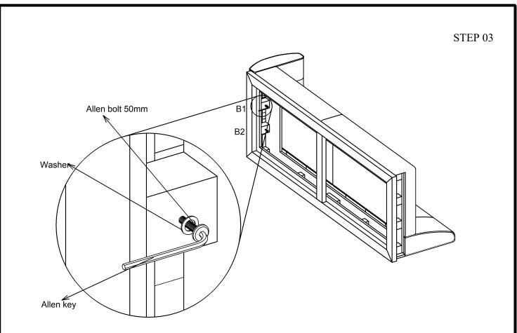
Fix the Part-B with last assemble part by washer and allen bolt M8x50mm with allen key at position B1& B2 as shown in Fig.
