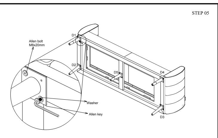
Fix Part-D with last assemble part by allen bolt M8x20mm using Allen key at position D1,D2,D3,D4 & D5 as shown in Fig. STEP 06
